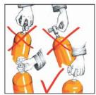
Tragarten: am Ventil, nie am Handrad. Lifting: by the valve, never by the handwheel.
